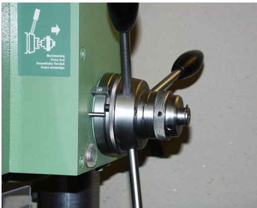
Picture 2. Inserted coupling
